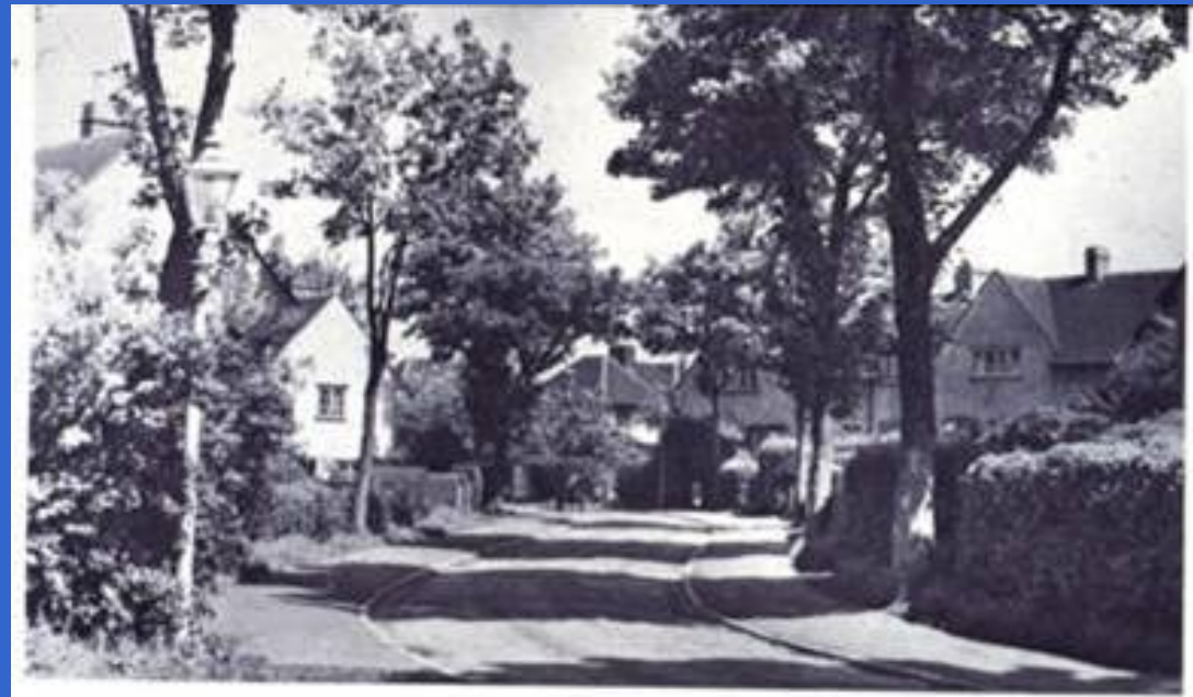
Fig. 8a. Rushby Mead, Letchworth. This street captures the originally intended balance between nature and architecture, with the plain gables rising at unusual angles to the road line to give shape and direction to the space. The architects did not usually employ the S-curve, preferring to be more subtle, but this street happened to follow an old stream bed, and so was a response to a natural feature.
